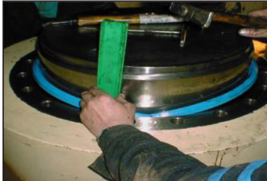
Split seal design with the wipers protecting the hydraulic system.
